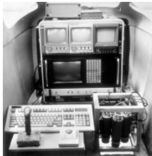
Figure 4. Airborne three-camera video system employed for detection of aquatic macrophytes in Texas.
