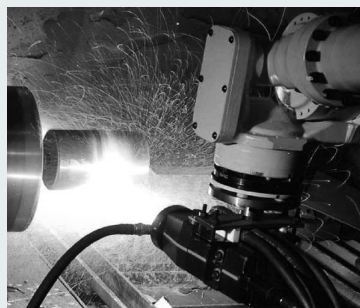
(Left) Steel matrix composites. (Right) Thermal spray coating process.
