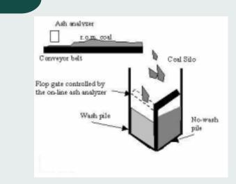
Physical segregation of coal using on-line analyzer (Source: Ganguli, R., Yingling, J.C., Zhang, J., Sottile, J., and Kumar, R., 1999, "Optimal Control of Coal Segregation Using on-line Quality Analyzers," Mining Engineering, April, pp. 41-48.)
