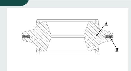
The disc cutter body material (A) surrounding a hard material insert (B) will be HIPped in one step by the CastCon Process.
