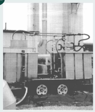
A mobile ASH system such as the one shown above will be used for cyanide recovery/destruction.
