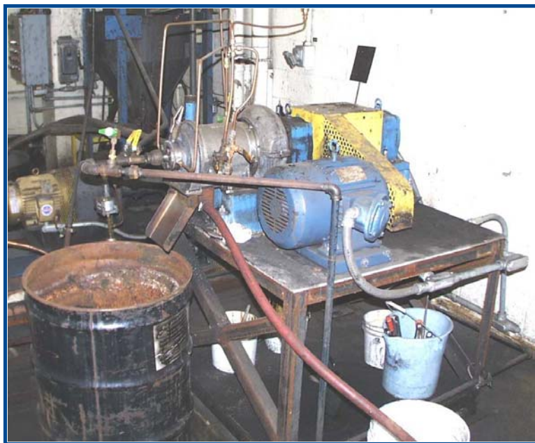
This 6-inch, screen-bowl centrifuge was used by Dr. Wen, U.S. Department of Energy, for POC testing of the GranuFlow Technology.
