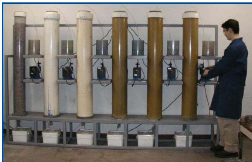
Columns for simulating heap leaching.
