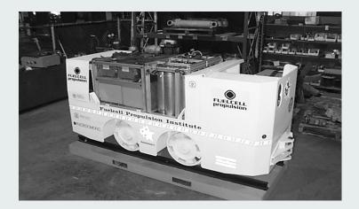
Fuel cells can give mining locomotives such as the one above the mobility and energy capacity of a diesel vehicle but the environmental characteristics of electric vehicles.
