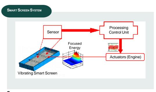
Conceptual design of a closed loop control system for a Smart Screen System.
