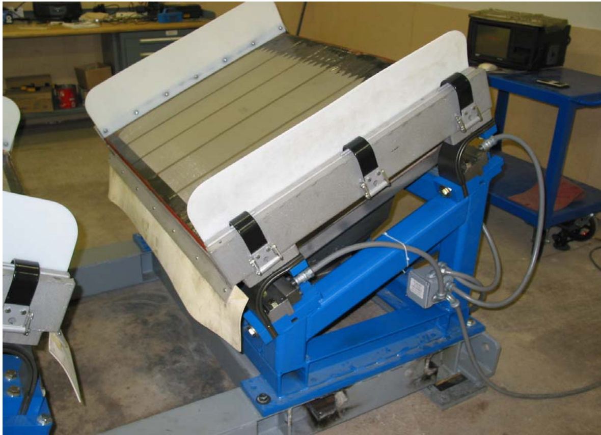
Figure 1 PZT system setup on field-ready supporting structure
