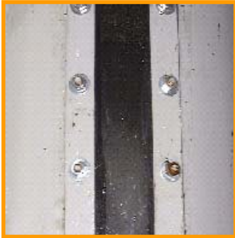
Viewing window in the CrossFlow unit showing upper (coal) and lower (rock) particle separation.
