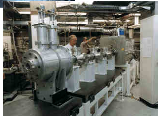
Linear magnetic-transport experiment. Recent scaled experiments at Lawrence Livermore National Laboratory tested the injection, matching, and magnetic transport of a potassium-ion beam.
