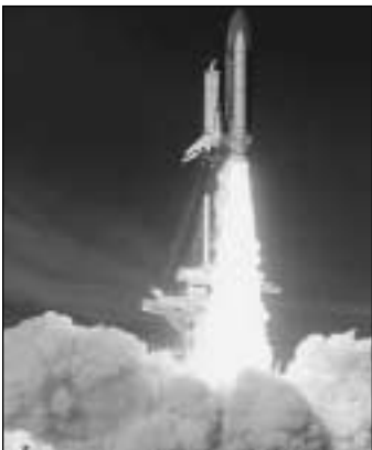
NASA uses liquid hydrogen to launch its space shuttles and hydrogen fuel cells to provide them with electricity
