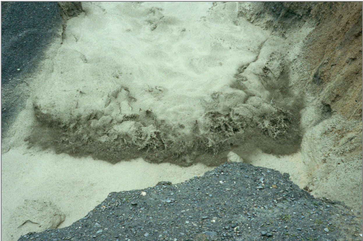
Figure 3. Photo of surge front on June 15, 1990. Note spray of ejected particles from surge front, especially at right margin (left bank). Width of surge is 20 m (66 ft). Photo by K.M. Scott.
