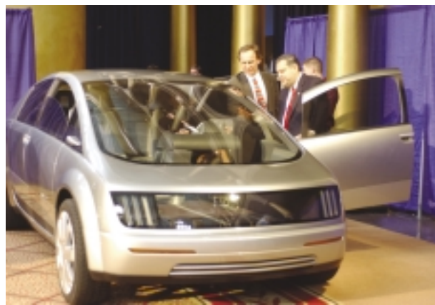
Secretary of Energy Abraham examining a hydrogen powered vehicle at the "Clean Energy for the 21st Century" exhibit. General Motor's Hy-Wire is a combination of hydrogen propulsion and drive-by-wire controls. Vehicles that run on hydrogen fuel produce only water, not exhaust fumes, thereby reducing pollution and reliance on fuel from other countries.
