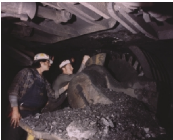
Miner is inspecting double ranging drum shearer.
