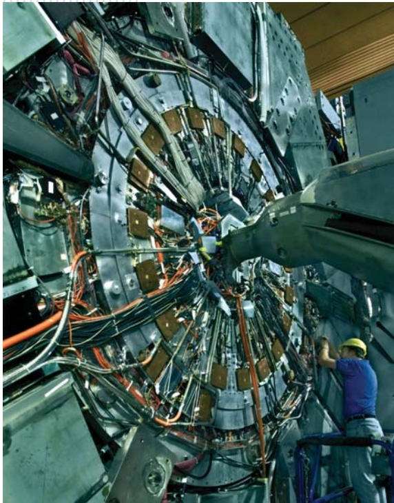
Technician at the B Factory's huge BABAR detector system at the Stanford Linear Accelerator Center. BABAR is a 1,200 ton detector system that can sift through the 238 million beam crossings that will occur every second in the B Factory and analyze the three to four events that can best be studied for charge-conjugation/parity.
