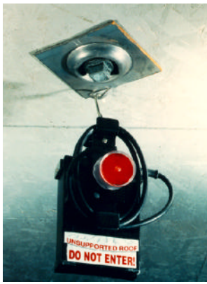
Figure 1.—Rechargeable roof hazard alert module (4-V).
