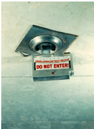
Figure 2.—Disposable magnetic-mount roof hazard alert module (9-V).
