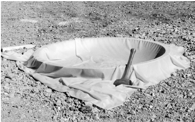
Figure 5.—Density frame covered with natural latex rubber sheeting.
