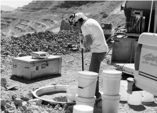
Figure 4.—Frame for in situ density tests.
