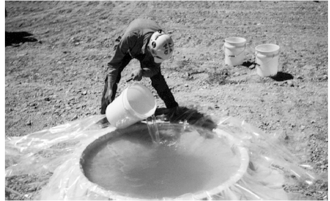
Figure 6.—Density pit lined with polyethylene sheeting and filled with water.
