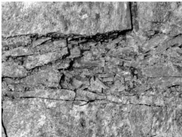
Figure 6. Disrupted zone formed by shearing within 4-cm-wide zone of closely spaced mining-induced extension fractures in stope walls.
