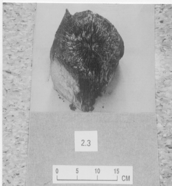
Figure 2.—Sample 2.3 (partially charred wood-crib block) from set 2.
