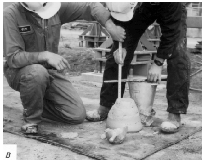
Consistency of total tailings paste backfill at different slumps. A, 27-cm slump; B, 13-cm slump.
