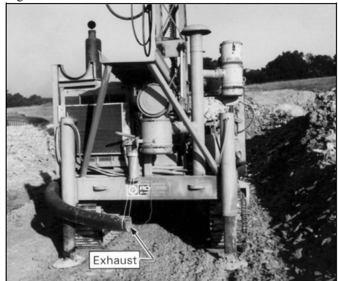
No visible dust in the exhaust from a drill equipped with the water-trickle system.
