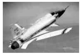
movable canards, enhanced maneuvering and cruise capabilities at transonic speeds. That phase was flown with the No. 1 X-29 aircraft and ended in 1989. NASA's high-angle-of-attack research program with X-29 No. 2 ended in 1991 and demonstrated that the aircraft design had better-than-expected control and maneuverability at angles of attack up to 45 degrees.
