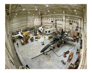
door that is 40 feet high and 126 feet wide. Test bays four and five together are 125 feet wide by 99 feet deep. The door to test bay six is 40 feet high and 100 feet wide. Test bay six is 97 feet wide by 99 feet deep. A full-height wall separates test bays five and six.
