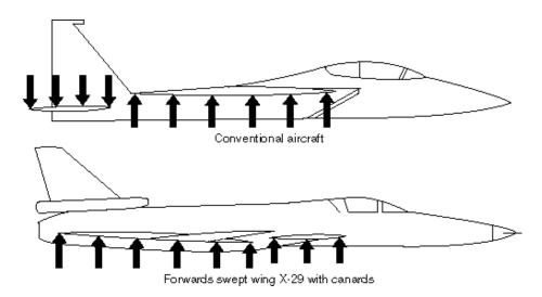
X-29 - designed with relaxed static stability to achieve less drag, more maneuverability, increased fuel efficiency. Arrows in upper illustration indicate drag-producing opposing downward forces on rear stabilizers to achieve stability. X-29 canards share lifting loads, reducing drag.
