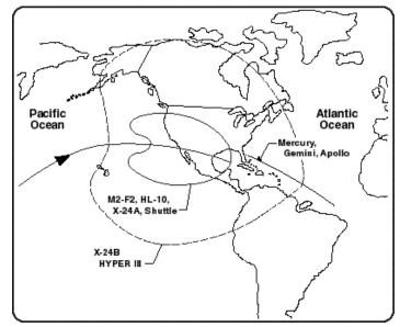
Orbital entry footprints (lateral and longitudial maneuverability) of lifting bodies and spacecraft. (Note the very small area for the Mercury, Gemini, and Apollo capsules as compared with the lifting bodies and the Space Shuttle.)
