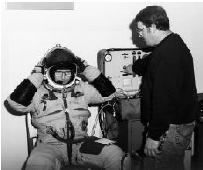
An ER-2 pilot is assisted into a full pressure suit in preparation for flight. The suit ensures survivability at high altitude in the event of aircraft cabin depressurization.
