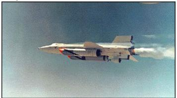
X-15A-2 (with ablative coating and external tanks) in which Pete Knight set the unofficial world speed record. NASA photo EC68 1899
