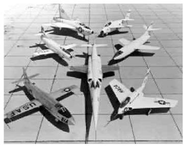
NASA Photo E-2889. NACA Research Aircraft - Bell X-1A, D-558-1, SF-92A, X-5, D-558-II, X-4, and X-3.
