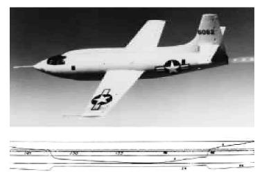
Photo E60-6204A. X-1 in flight with copy of "mach jump" paper tape data record of the first supersonic flight.
