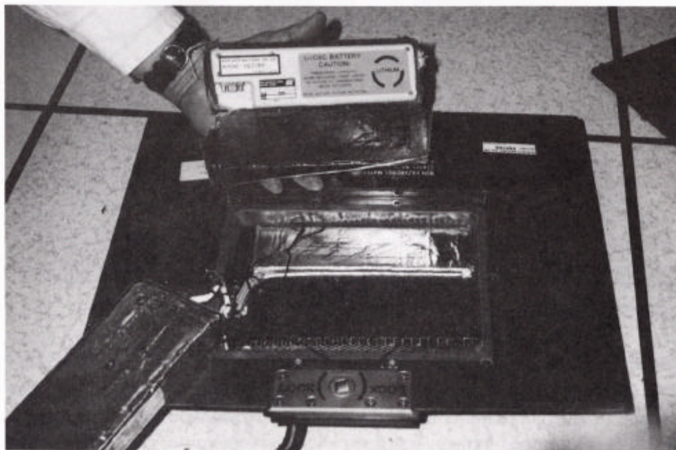
Figure 5. DFIRS battery (unwrapped) shown above installed battery
