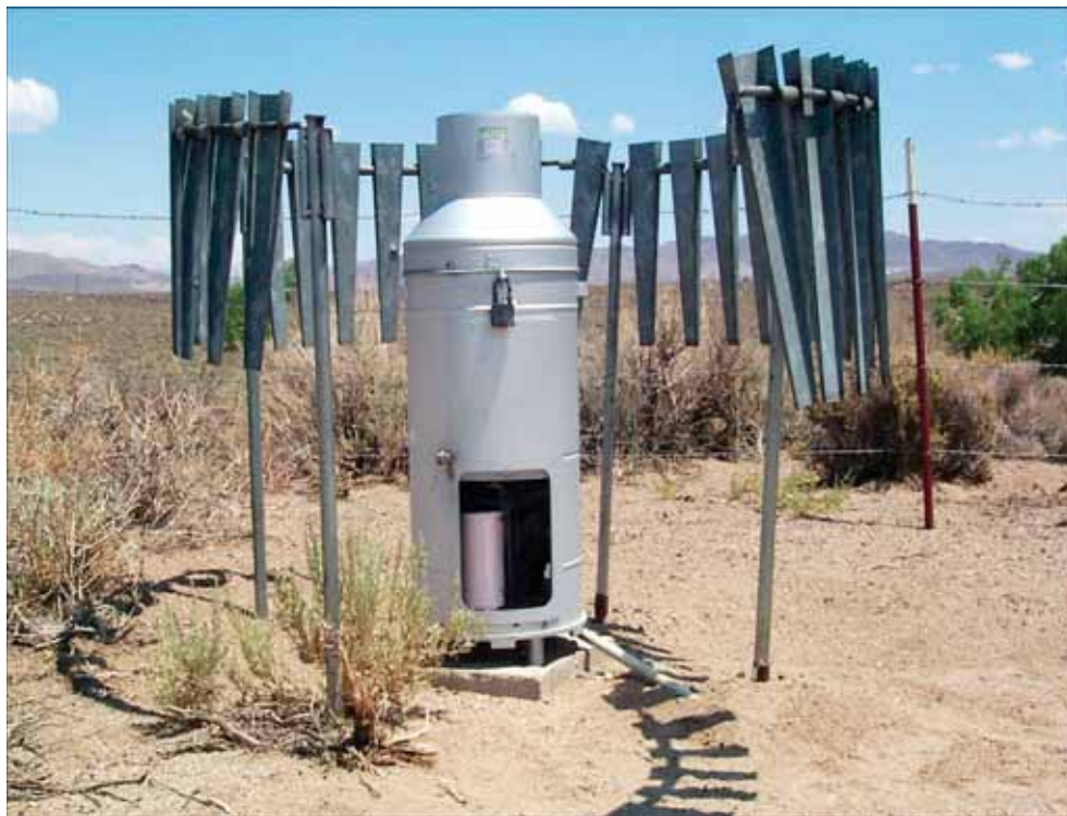
Figure 2. Belfort 5-780 precipitation gage, at site NV03, showing Belfort rotating chart.
