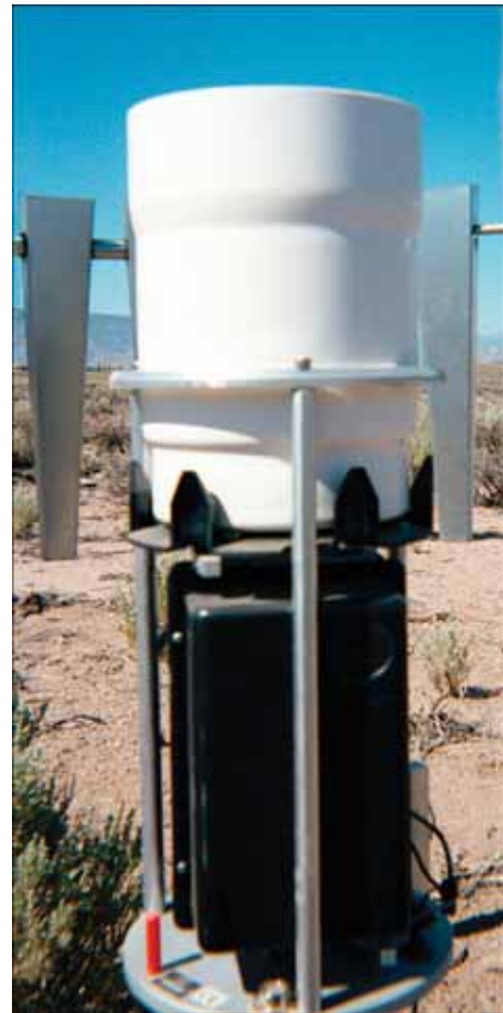
Figure 3. (A) OTT PLUVIO precipitation gage with stainless steel housing, at site NV03. (B) OTT PLUVIO precipitation gage with stainless steel housing removed showing collection bucket and data logger.
