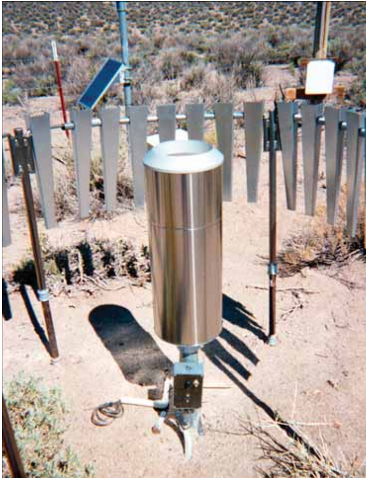
Figure 3. (A) OTT PLUVIO precipitation gage with stainless steel housing, at site NV03. (B) OTT PLUVIO precipitation gage with stainless steel housing removed showing collection bucket and data logger.
