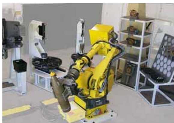
A ROBOTIC DISASSEMBLY system, like the one shown here, enables safe dismantlement of aging munitions.
