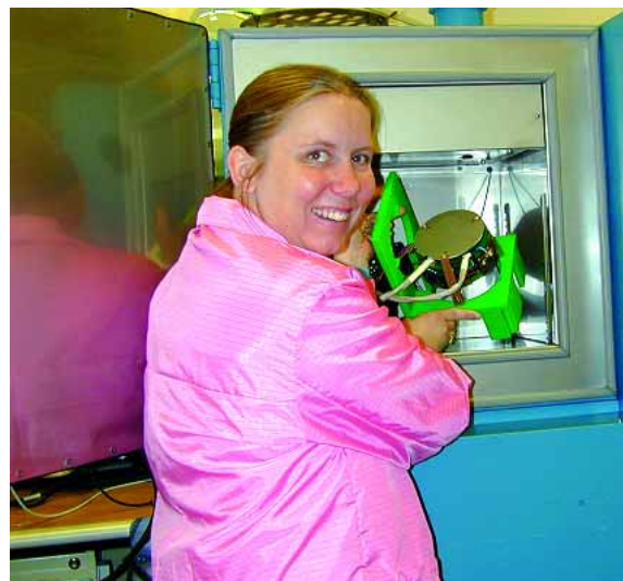
TESTING — Molly McCandless (2300) prepares a W76-1 arming and fuzing system prototype for temperature testing.
