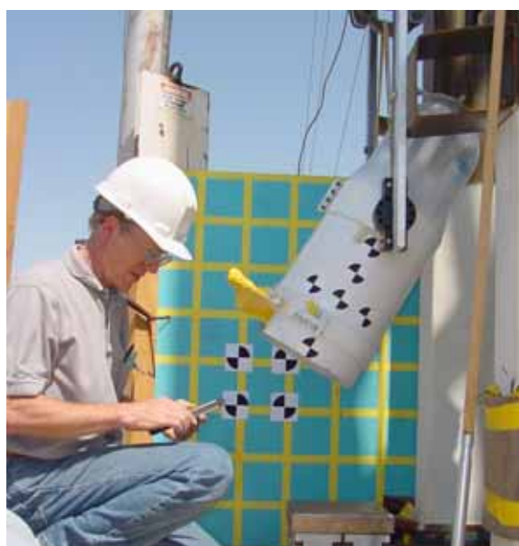
PREPARING for a W80-3 drop test at Sandia's Drop Tower test facility. The test, done with the ASCI program, is part of the ongoing W80-3 Life Extension Program.
