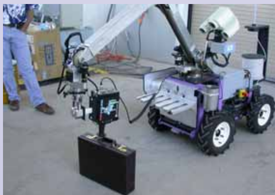
ROBOHOUND interrogates a briefcase contaminated with explosives during an experimental test.
