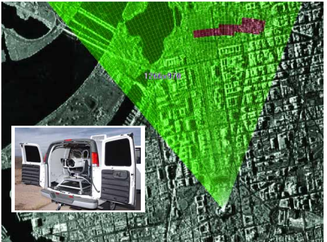
DEPICTION of how the Ares lidar could be deployed in urban areas for detection of biological material releases.
