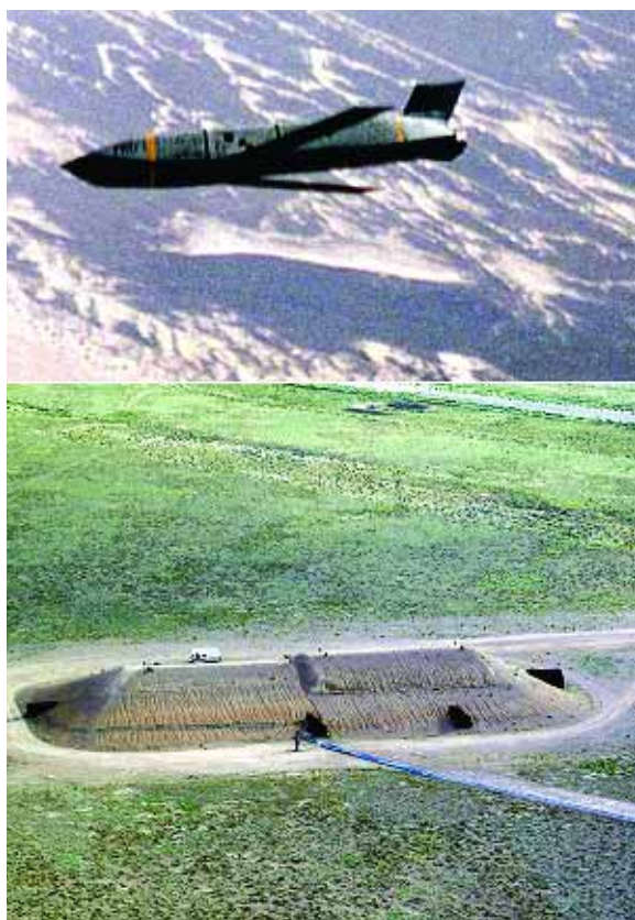
JOINT AIR-TO-SURFACE MISSILE flight tests being conducted at Sandia's Tonopah Test Range in Nevada. Top photo shows missile in flight; bottom photo shows bunker target.
