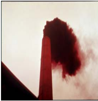
Smoke stacks like this one create emissions that decrease visibility in their surrounding areas. The BART requirements would control those emissions to improve visibility.
