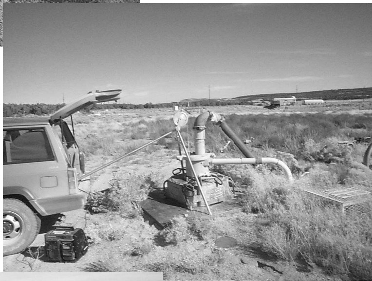
Water level being measured in water-supply well U-20 WW on Pahute Mesa, 1999 (Photograph by Gary Otto, U.S. Geological Survey).
