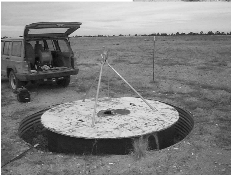
Water level being measured in well U-19bj on Pahute Mesa, 1999 (Photograph by Gary Otto, U.S. Geological Survey).
