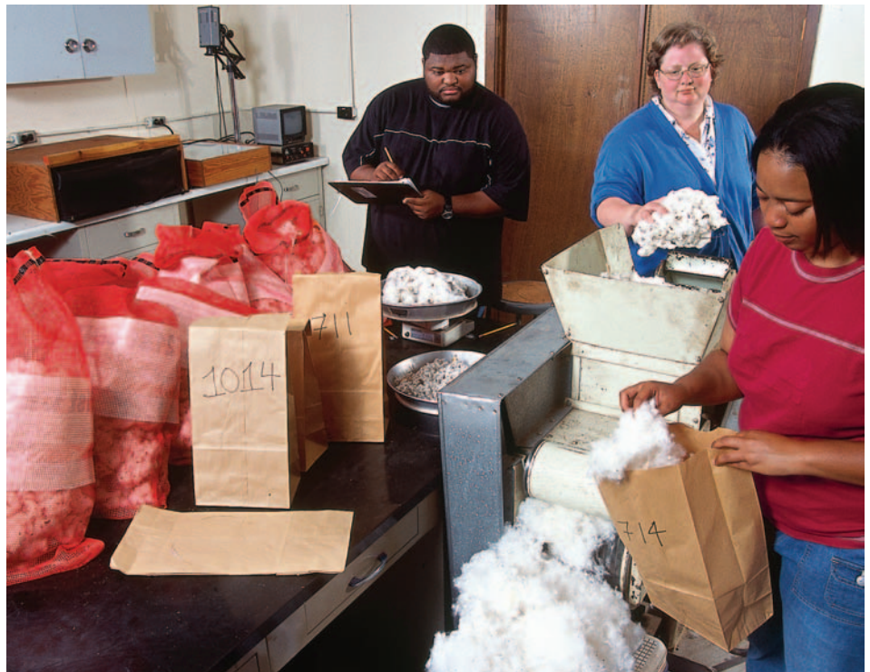
Biological science aid Jason Corbit (left) records cotton sample weights while Gretchen Sassenrath (center) and biological science aid Ebony Scott gin the seed cotton samples in preparation for fiber analysis at the USDA Agricultural Marketing Service classing office.
