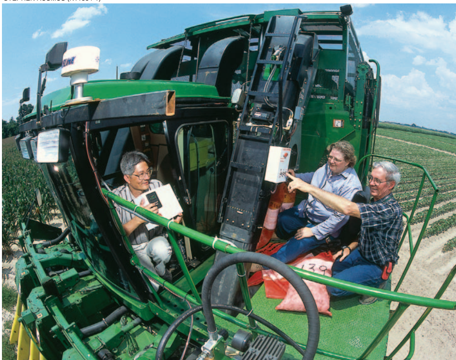
At ARS's Application and Production Technology Research Unit in Stoneville, Mississippi, (left to right) agricultural engineering professor Filip To, plant physiologist Gretchen Sassenrath, and technician Ray Adams perform final installation and testing of the automated sampling system on a cotton picker.
