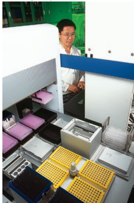
Technician Guilin Wang sets the conditions for operation of an automated robotic system for purifying DNA. High-quality DNA is required for spotting onto glass slides for microarray experiments.
