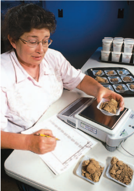
Technician Joyce Alloway weighs sections of dried soil cores before grinding and analysis for total carbon.
