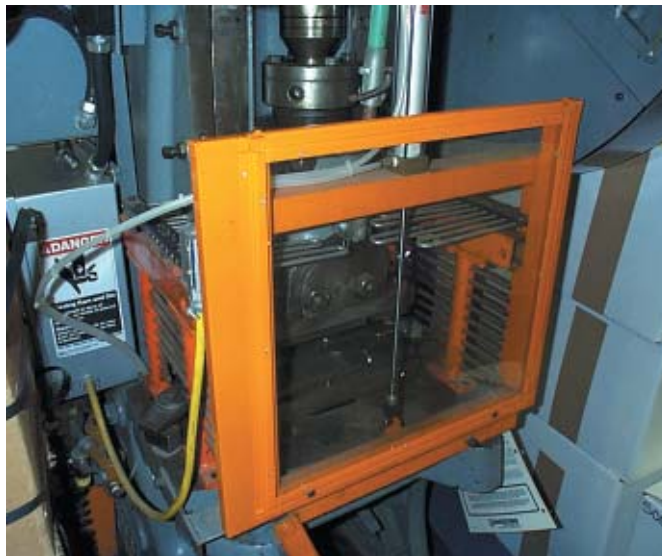
Physical guards keep operators from reaching into moving machine parts.
