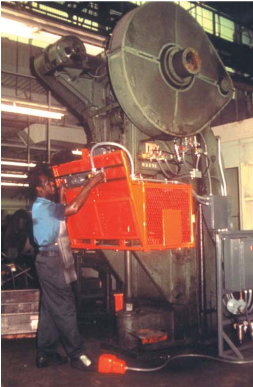
Machine guards on a power press protect a worker from amputations and other injuries.
