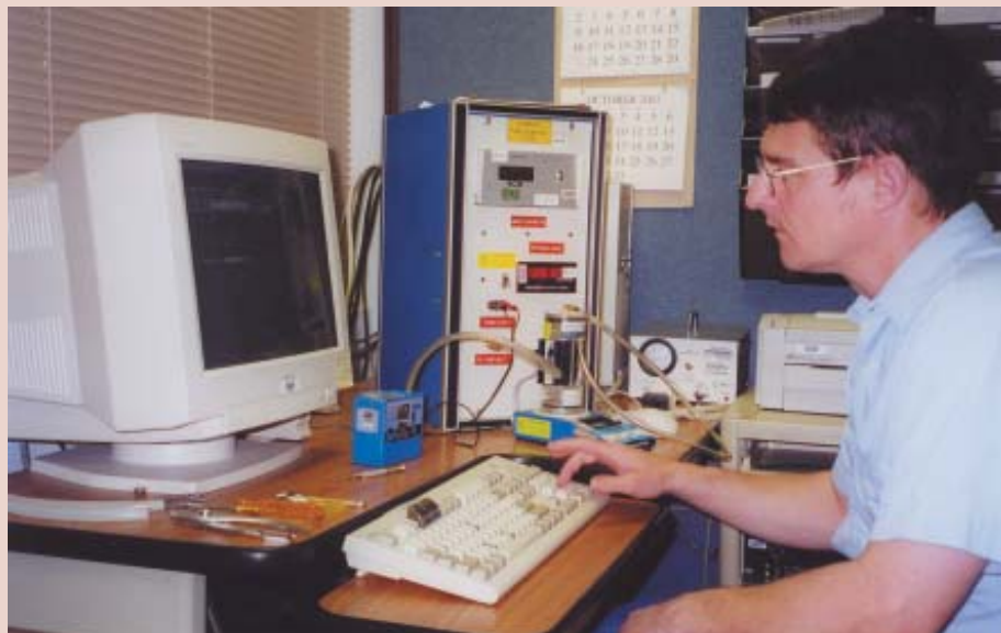
Engineering Technician Harry Rollyson calibrates an air sampling pump at an automated pump calibration station. Photo by Ray Feldman
