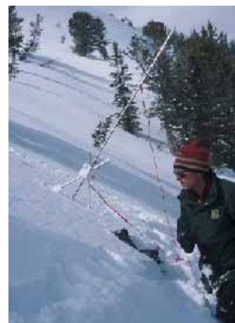
Geographer Karl Birkeland uses a new microsensor to determine spatial patterns of snow stability
