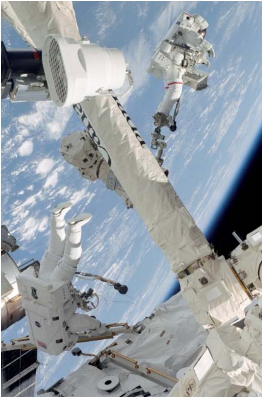
Oct. 12, 2002, astronauts David A. Wolf (left) and Piers J. Sellers, both STS-112 mission specialists, participate in the mission's second session of extravehicular activity (EVA). Wolf is anchored to a foot restraint on the International Space Station's (ISS) Canadarm2 while Sellers traverses along the airlock spur, a route used by spacewalkers to get from the Quest airlock on the station to the outpost's truss.
