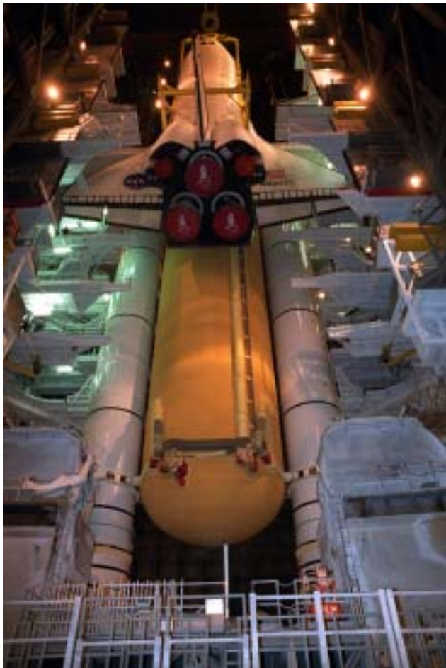
In the Vehicle Assembly Building, the orbiter Atlantis is lowered into position for mating to its external tank/solid rocket booster stack for launch on mission STS-104 July 12, 2001.
