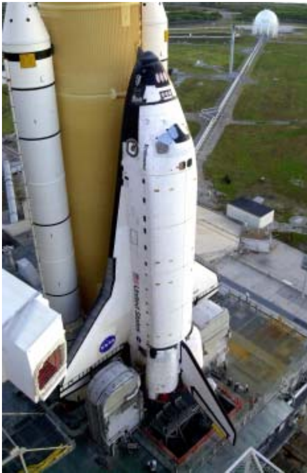
Space Shuttle Endeavour, with its stack of solid rocket boosters and external tank, sits on Launch Pad 39A for launch of STS-113. At lower left is the White Room, situated at the end of the orbiter access arm, which provides entry into the orbiter for the crew.
