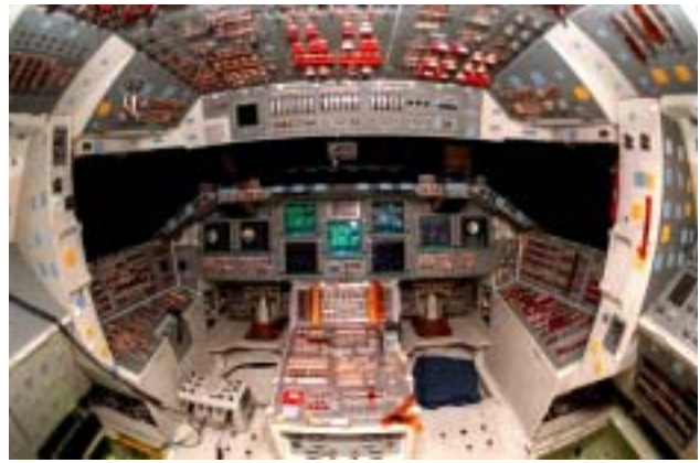
The "glass cockpit" provides easy-to-read, graphic portrayals of key flight indicators like attitude, altitude and speed.
