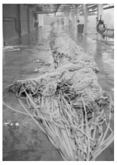
After the chutes are returned to the PRF following launch, a hanging monorail system is used to transport each parachute into a 30,000-gallon washer and then into a huge dryer heated with 140degree air at 13,000 cubic feet per minute.
