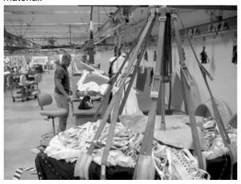
After the chutes are cleaned and repaired, they must be carefully packed into their bags (above) so they will deploy correctly the next time they are used. It takes about a week to pack a main canopy, for example.
