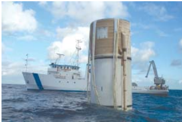
A retrieval ship arrives at a half-submerged solid rocket booster after a Shuttle launch. Divers will prepare the SRB under water to float horizontally and be towed back to Port Canaveral.
