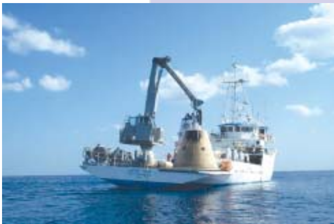
(Above left) The drogue chute is wound onto a reel on deck. (Left) The frustum is lifted from the water by a power block attached to the ship's deck crane.
