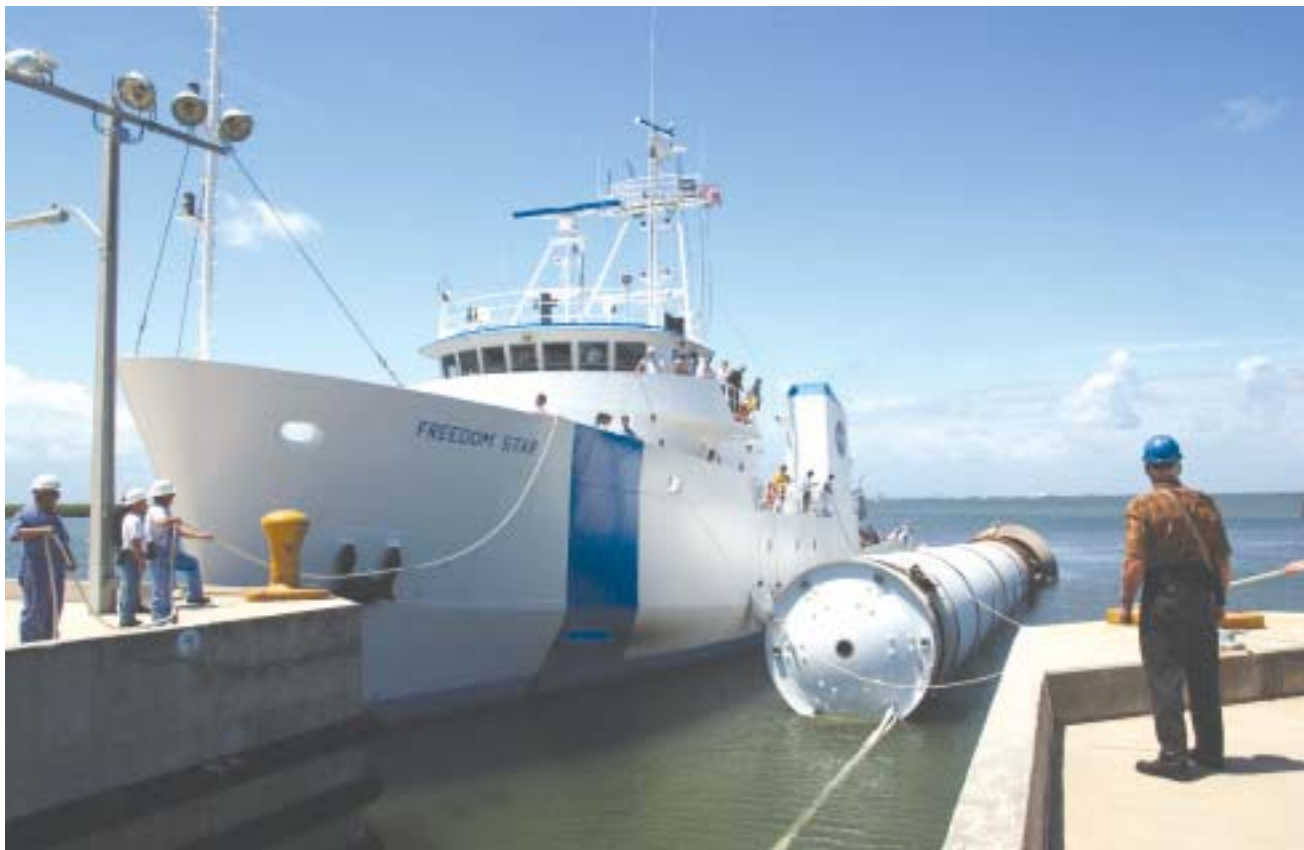
At Hangar AF, the booster is released from the ship. It will be towed to a position where Straddle-Lift cranes can lift it from the water and place it on a rail car for disassembly.
