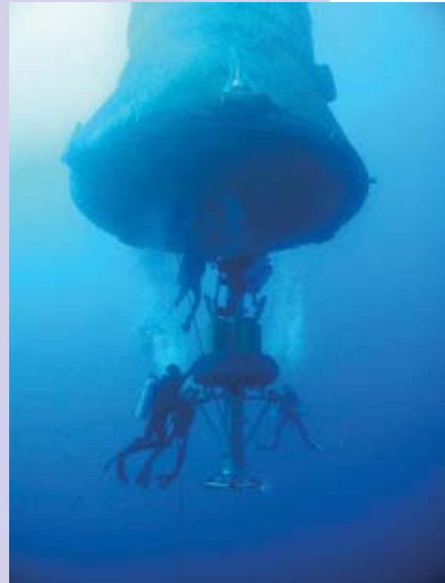
(Above) Divers insert an Enhanced Diver-Operated Plug into the booster nozzle, displacing the water and causing the booster to assume a semi-log or horizontal position.
