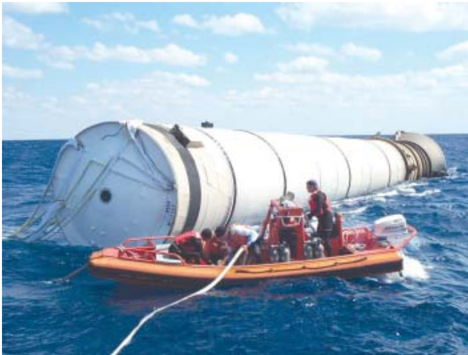
(Left) Divers attach tow lines to the floating booster.
