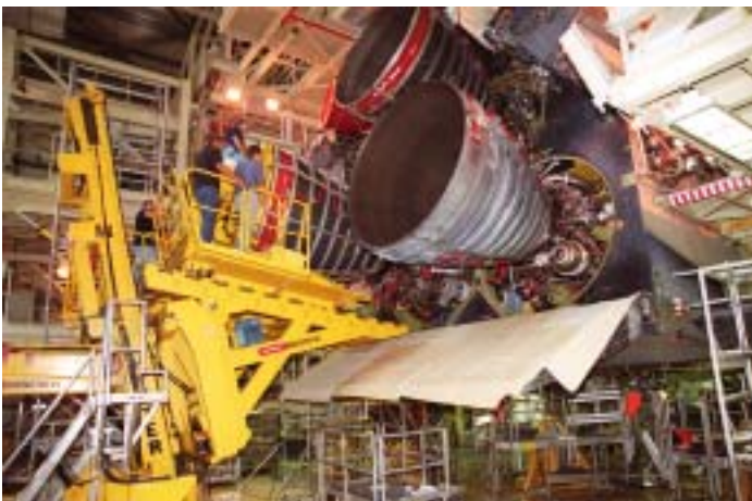
Using a crane, technicians in the SSMEPF install a new turbo-charged engine in the orbiter Atlantis.
