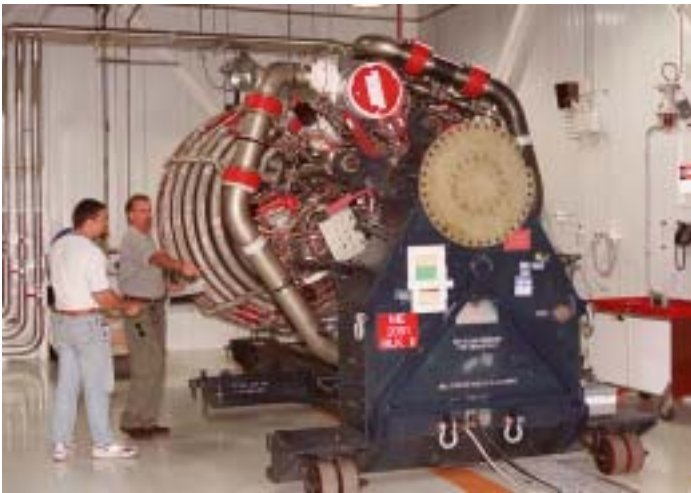
This Space Shuttle Main Engine contains 50,000 parts, of which 7,000 are tracked periodically for replacement.
