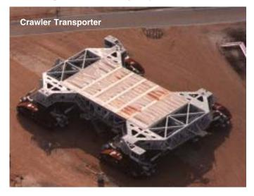
When the Shuttle orbiter has been mated to the external tank and solid rocket boosters, the CT lifts the mobile launcher with the Shuttle, and carries it to the launch pad using a laser guidance system on the crawler and a leveling system.
