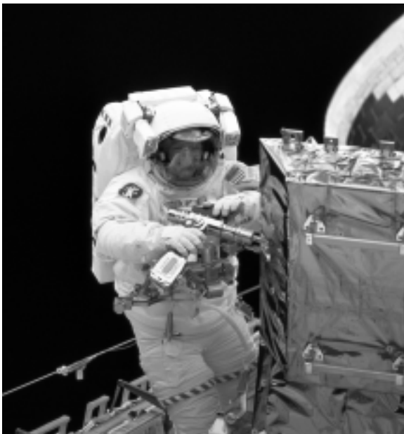
On a Hubble Servicing Mission (STS-103) in 1999, astronaut Claude Nicollier, mission specialist from the European Space Agency (ESA), works at a storage enclosure, using one of the Hubble power tools, during the second of three extravehicular activities (EVA).
