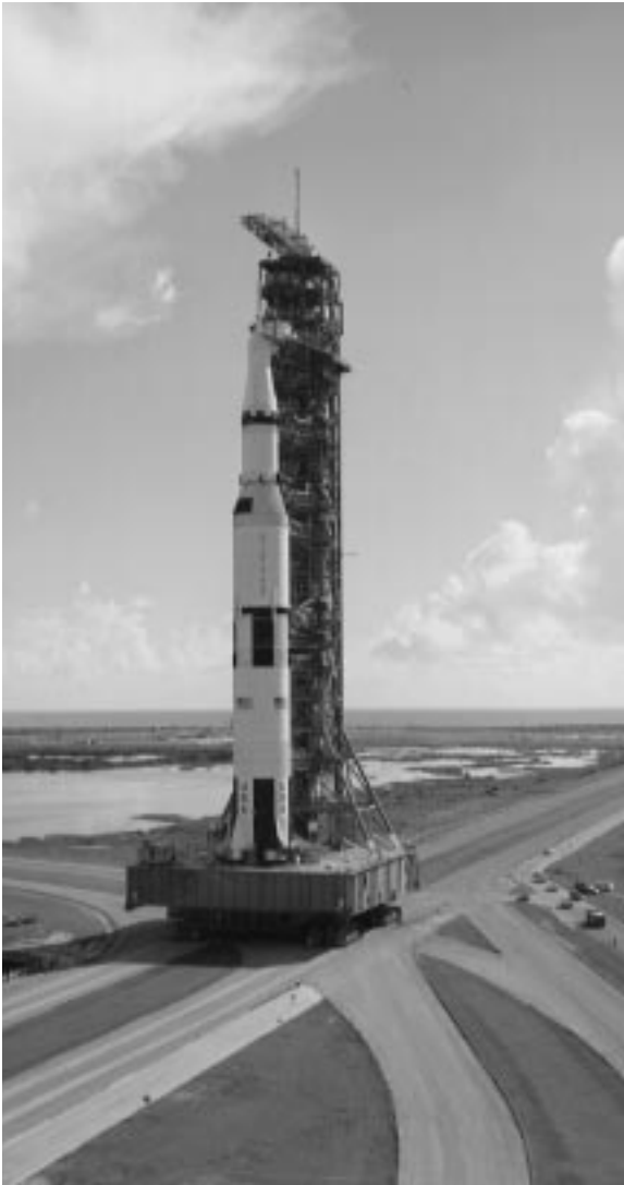
Apollo 17 heads for Pad A atop its giant Saturn V rocket for the last manned flight to the Moon. Riding a mobile launcher that towered well over 400 feet into the air, with a total weight on the crawler-transporter treads of over 18 million pounds, an Apollo/Saturn V vehicle in motion on the crawlerway was an awesome and unforgettable sight.
