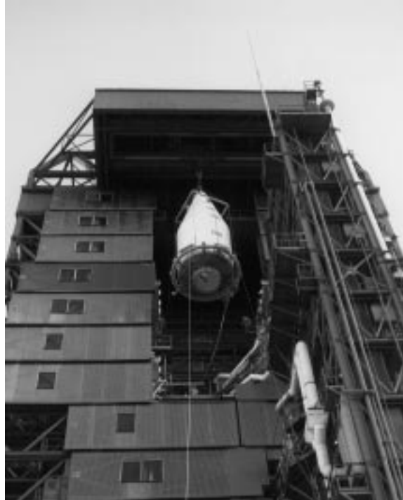
The overhead crane in the gantry on Pad B, Launch Complex 36, lifts a Centaur nose fairing toward the opening to the interior. Inside the fairing was a FLTSAT-COM military satellite spacecraft. Once inside the gantry the nose fairing was mated with the Atlas/Centaur.
