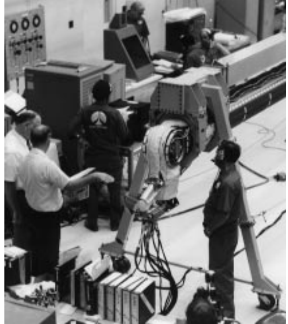
A Shuttle remote manipulator arm undergoes testing by engineers and technicians inside one of the Spaceport's clean rooms before being installed in the cargo bay of an orbiter. The mechanism, built in Canada, helps astronaut crews handle payloads in space.
