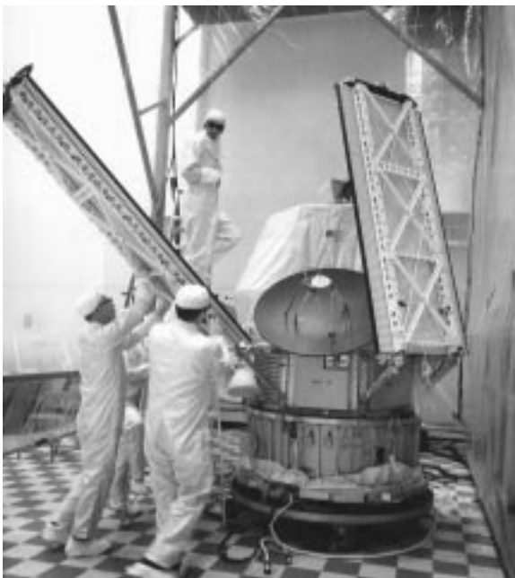
Technicians install a solar panel on Mariner 8, launched on May 8, 1971. It was half of a twin launch of scientific spacecraft, planned to survey Mars from orbit. Mariner 9 reached the "Red Planet" next November 13, in the middle of a planet-wide dust-storm. It waited it out in orbit, then provided the first complete photographic record of the spectacular Martian surface.
