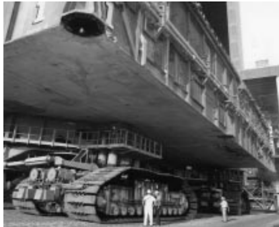
Spaceport workers are dwarfed by the massive tracks of a crawler-transporter as it carries a mobile launcher platform and a Space Shuttle vehicle (not visible atop the platform) from the Vehicle Assembly Building to the launch pad. Space Shuttle launch operations require experience and skills found nowhere else in the world.
