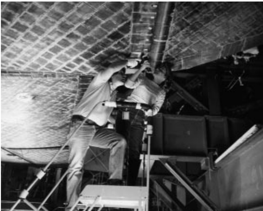
Readying a Space Shuttle orbiter for flight is an exacting job. Here, workers inspect the tiled underside of the orbiter Discovery during checkout and refurbishment operations inside the Orbiter Processing Facility.
