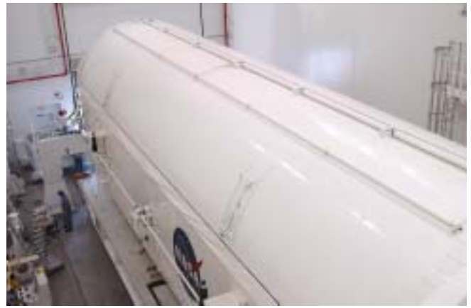
The canister is lowered onto its receiving pedestals.
