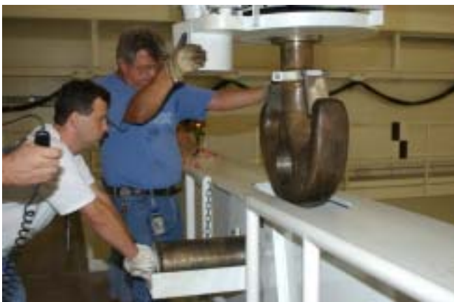
Technicians prepare to install a huge locking pin through the spreader bar and crane hook. The bar is used to rotate the payload canister in the CRF.
