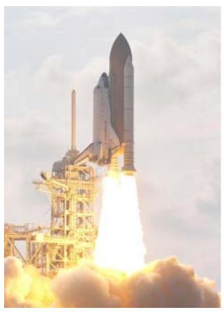
Space Shuttle Endeavour clears the lightning mast and attached catenary wire as it hurtles into space on mission STS-111 to the International Space Station, June 5, 2002. The mast and wire provide the primary lightning protection system for the orbiter while it is on the pad. Mission STS-111 is the 18th flight of Endeavour and the 110th flight overall in NASAis Space Shuttle program.
