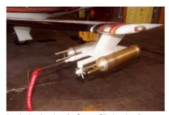
Attached to the wing of a Cessna Ciltation aircraft are cloud physics probes that measure the size, shape and number of ice and water particles in clouds. The plane is also equipped with field mills, used to measure electric fields. The plane is being flown into anvil clouds in the KSC area as part of a study to review and possibly modify lightning launch-commit criteria.
