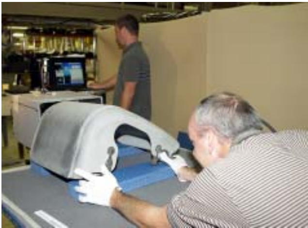
United Space Alliance worker Dan Kenna (right) positions a Reinforced Carbon-Carbon panel on the table to perform flash thermography. In the background, Paul Ogletree observes the monitor.
