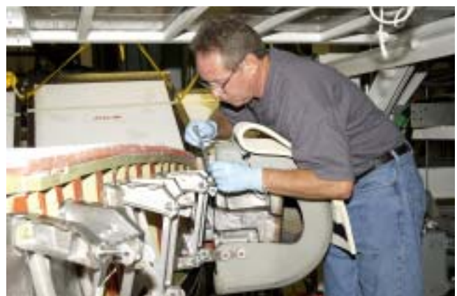
United Space Alliance worker Mike Hyatt attaches a Reinforced Carbon-Carbon (RCC) panel onto the leading edge of the wing of the orbiter Atlantis, which is being prepared for Return to Flight on mission STS-114.
